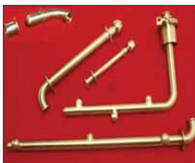
Figure 3: Commonly used CIP spray device types
