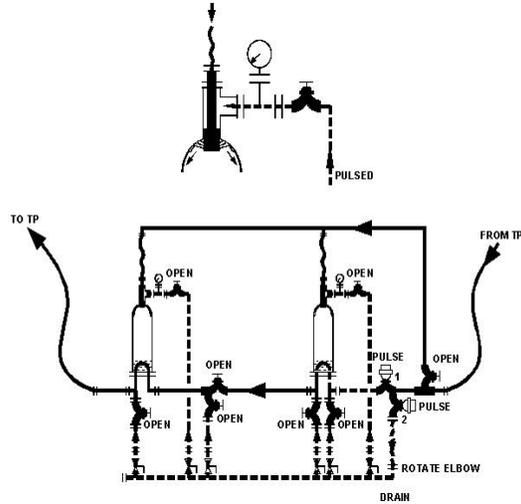
The Tube Spray was selected to permit the inlet nozzle tee branch to be cleaned by reverse flow through the VENT/COND lines. The CIP Procedure included the following steps.
