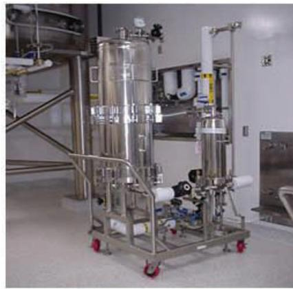
**Two Filter Housings of like size cleaned in parallel (left) and of unlike size cleaned in parallel (right)**
