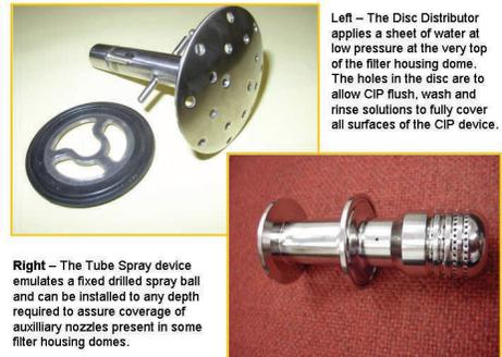
Left – The Disc Distributor applies a sheet of water at low pressure at the very top of the filter housing dome. The holes in the disc are to allow CIP flush, wash and rinse solutions to fully cover all surfaces of the CIP device.
