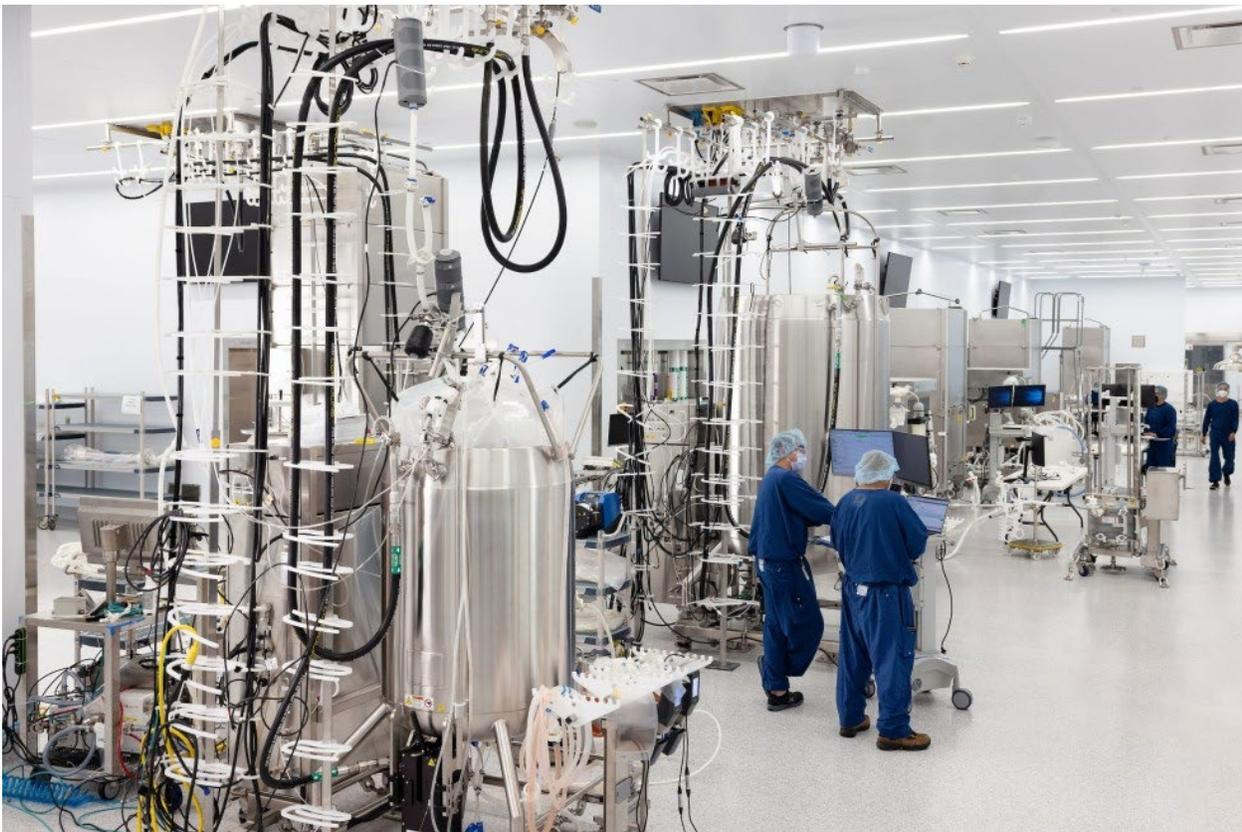
Monitoring conditions in the bioreactor to promote optimal cell growth.
